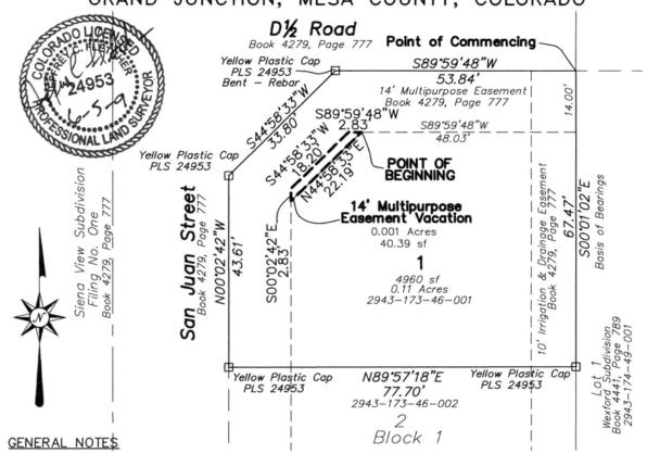
Basis of bearings is the East line of the Lot 1, Block 1, Siena View Subdivision, Filing No. One, as recorded in Book 4279, Page 777, which bears South 00 degrees 01 minutes 02 seconds East, a distance of 67.47 feet, established by observation of the MCGPS control network, which is based on the NAD 83 for Horizontal and NAVD 88 for Vertical Information. Both monuments on this line are Lot Corners, as shown on the face of said plat of Siena View Subdivision, Filing No. One.
